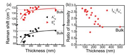
Figure 6. Thickness dependent Raman spectra of strain-free  $Bi_2Se_3$  nanoribbons. (a) Raman shift of  $A^1_{1g}$  and  $E^2_g$  modes *versus* thickness. The black (red) solid line is fitting curve of  $A^1_{1g}$  ( $E^2_g$ ) mode. (b) Ratio of intensities  $I_{A^1_{1g}}/I_{A^2_{1g}}$  versus thickness. The bold lines indicate the corresponding value of  $Bi_2Se_3$  bulk material from ref 31.
