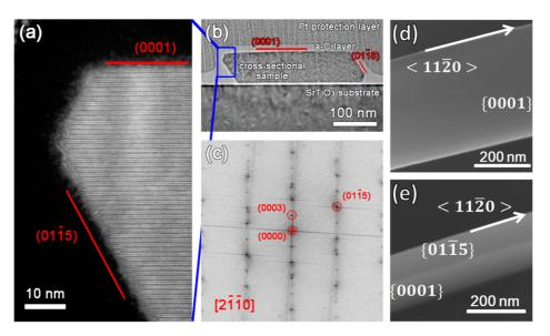
Figure 1. Characterization of as grown  $Bi_2Se_3$  nanoribbons. (a) High resolution HAADF-STEM image, (b) TEM image, and (c) the corresponding FFT pattern of (a) from a cross-sectional sample of  $Bi_2Se_3$  nanoribbon. High magnification SEM image of  $Bi_2Se_3$  nanoribbon (d) with the {0001} surface and (e) with the {0115} surface lying on the substrate.
